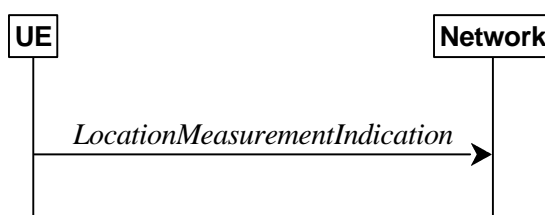
Figure 5.5.5.1-1: Location measurement indication
