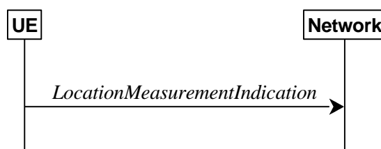
Figure 5.5.5.1-1: Location measurement indication
