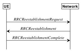
Figure 5.3.7.1-1: RRC connection re-establishment, successful
