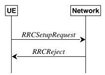
Figure 5.3.3.1-2: RRC connection establishment, network reject
