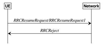
Figure 5.3.13.1-5: RRC connection resume, network reject
