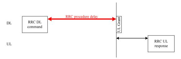
Figure 12.1-1: Illustration of RRC procedure delay
