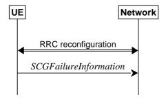
Figure 5.7.3.1-1: SCG failure information
