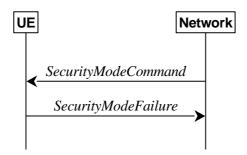
Figure 5.3.4.1-2: Security mode command, failure
