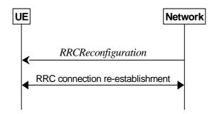
Figure 5.3.5.1-2: RRC reconfiguration, failure
