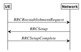
Figure 5.3.7.1-2: RRC re-establishment, fallback to RRC establishment, successful
