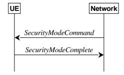
Figure 5.3.4.1-1: Security mode command, successful
