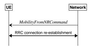
Figure 5.4.3.1-2: Mobility from NR, failure
