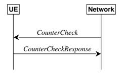
Figure 5.3.6.1-1: Counter check procedure
