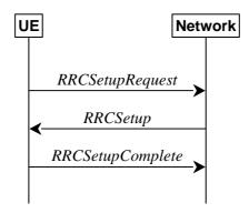
Figure 5.3.3.1-1: RRC connection establishment, successful
