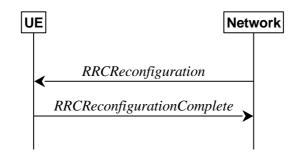
Figure 5.3.5.1-1: RRC reconfiguration, successful
