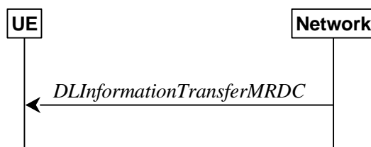
Figure 5.7.1a.1-1: DL information transfer MR-DC
