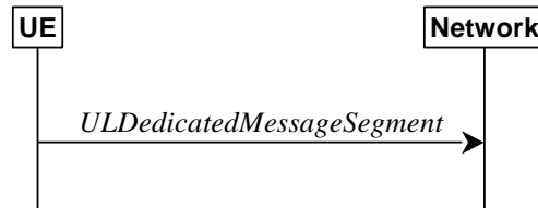
Figure 5.7.7.1-1: UL message segment transfer
