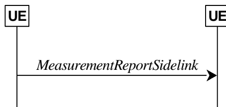
Figure 5.8.10.5.1-1: NR sidelink measurement reporting
