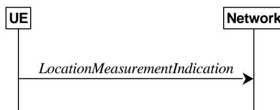
Figure 5.5.5.1-1: Location measurement indication
