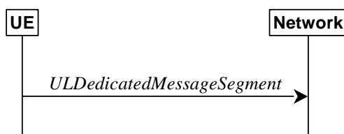
Figure 5.7.7.1-1: UL message segment transfer
