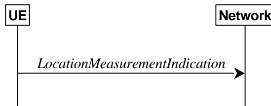
Figure 5.5.5.1-1: Location measurement indication
