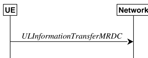
Figure 5.7.2a.1-1: UL information transfer MR-DC
