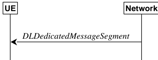
Figure 5.7.6.1-1: DL message segment transfer
