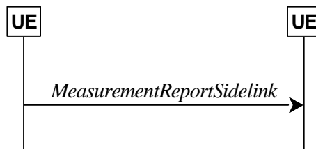
Figure 5.8.10.5.1-1: NR sidelink measurement reporting
