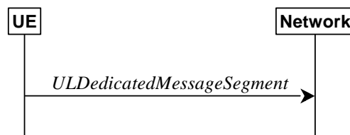
Figure 5.7.7.1-1: UL message segment transfer
