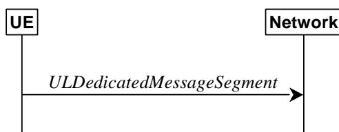
Figure 5.7.7.1-1: UL message segment transfer
