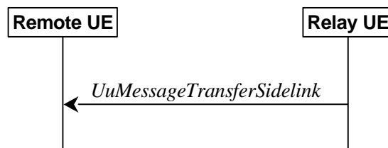
Figure 5.8.9.9.1-1: Uu message transfer in sidelink
