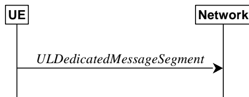
Figure 5.7.7.1-1: UL message segment transfer
