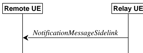
Figure 5.8.9.8.1-1: Notification message in sidelink
