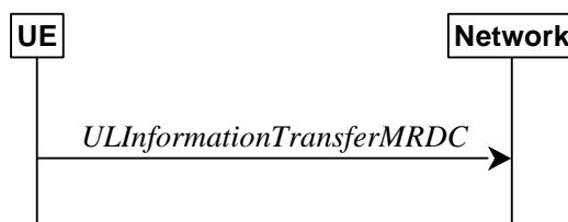
Figure 5.7.2a.1-1: UL information transfer MR-DC
