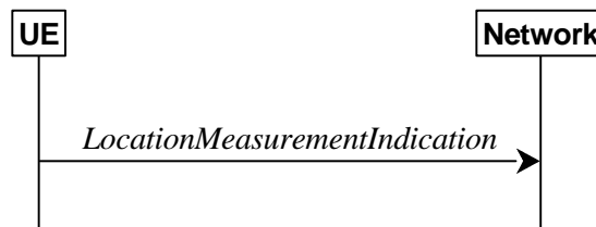
Figure 5.5.5.1-1: Location measurement indication
