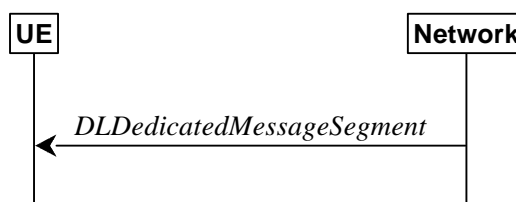
Figure 5.7.6.1-1: DL message segment transfer
