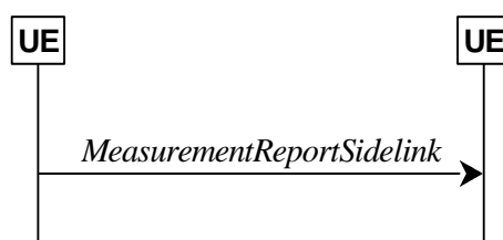
Figure 5.8.10.5.1-1: NR sidelink measurement reporting
