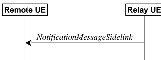
Figure 5.8.9.8.1-1: Notification message in sidelink
