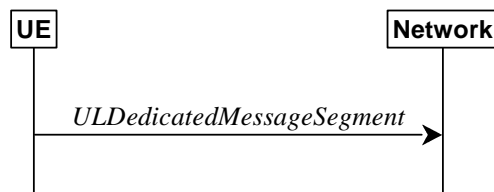
Figure 5.7.7.1-1: UL message segment transfer
