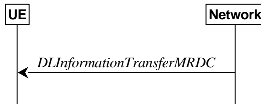
Figure 5.7.1a.1-1: DL information transfer MR-DC
