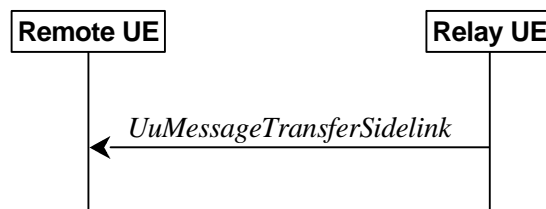
Figure 5.8.9.9.1-1: Uu message transfer in sidelink
