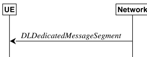
Figure 5.7.6.1-1: DL message segment transfer
