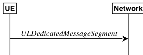
Figure 5.7.7.1-1: UL message segment transfer
