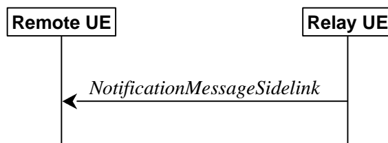
Figure 5.8.9.8.1-1: Notification message in sidelink
