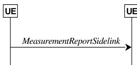
Figure 5.8.10.5.1-1: NR sidelink measurement reporting
