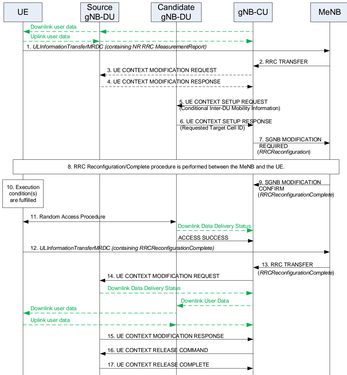
Figure 8.2.2.3-1: Inter-gNB-DU Conditional PSCell Change using MCG SRB without MN negotiation in EN-DC
