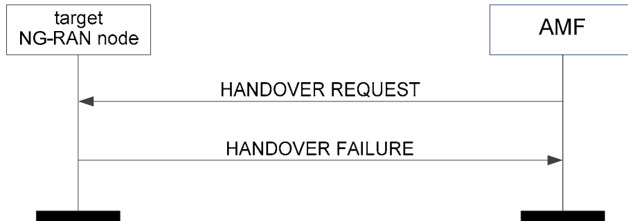
Figure 8.4.2.3-1: Handover resource allocation: unsuccessful operation
