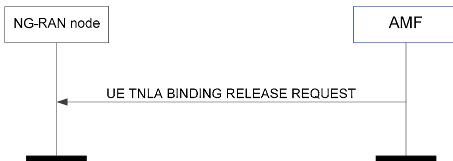
Figure 8.13.1.2-1: UE TNLA binding release request
