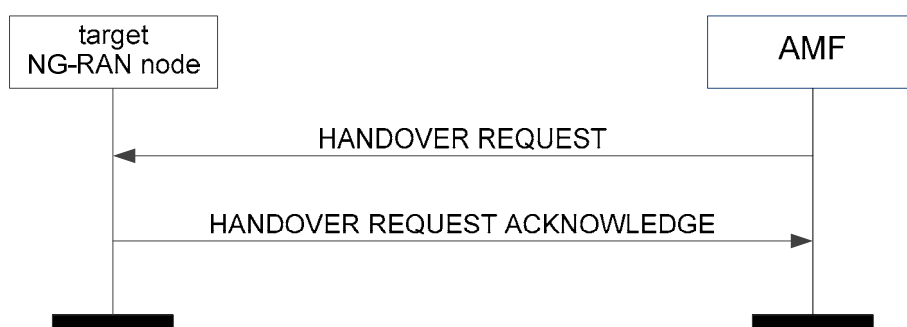
Figure 8.4.2.2-1: Handover resource allocation: successful operation
