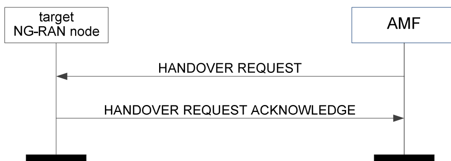
Figure 8.4.2.2-1: Handover resource allocation: successful operation
