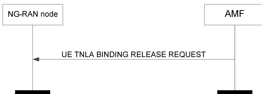
Figure 8.13.1.2-1: UE TNLA binding release request
