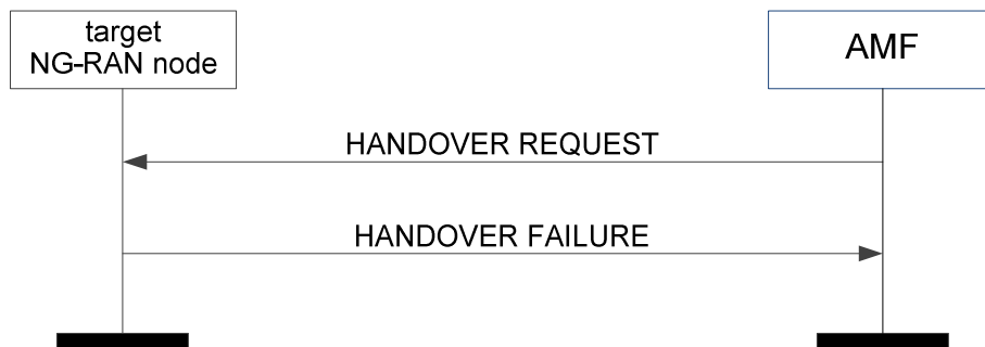
Figure 8.4.2.3-1: Handover resource allocation: unsuccessful operation
