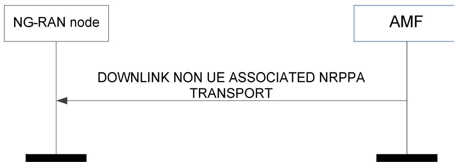
Figure 8.10.2.3-1: Downlink non UE-associated NRPPa transport
