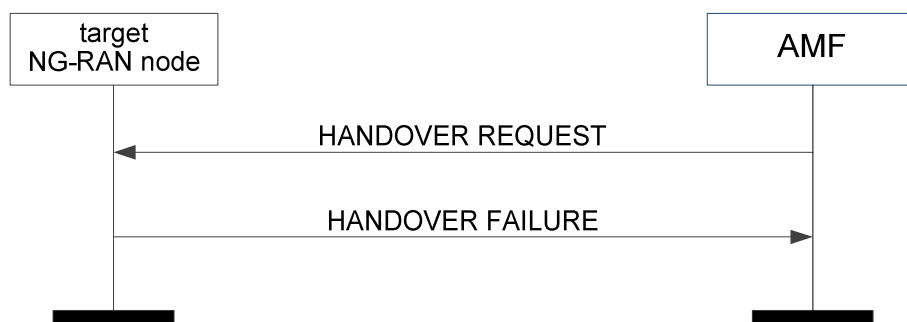
Figure 8.4.2.3-1: Handover resource allocation: unsuccessful operation
