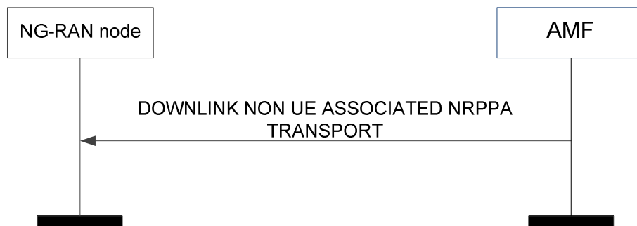
Figure 8.10.2.3-1: Downlink non UE-associated NRPPa transport
