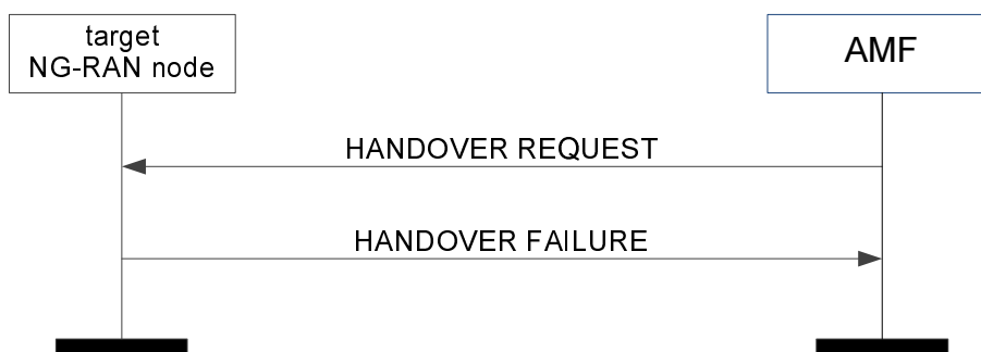
Figure 8.4.2.3-1: Handover resource allocation: unsuccessful operation
