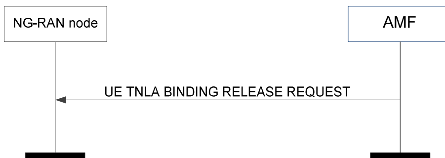
Figure 8.13.1.2-1: UE TNLA binding release request
