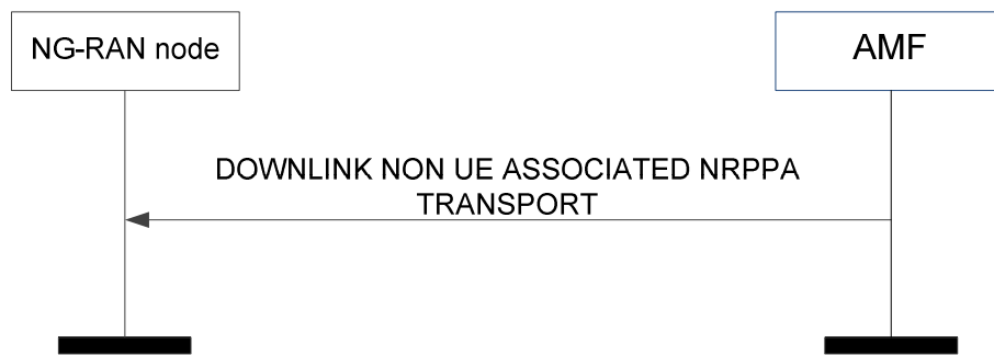
Figure 8.10.2.3-1: Downlink non UE-associated NRPPa transport
