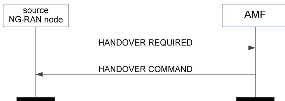
Figure 8.4.1.2-1: Handover preparation: successful operation
