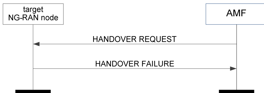
Figure 8.4.2.3-1: Handover resource allocation: unsuccessful operation
