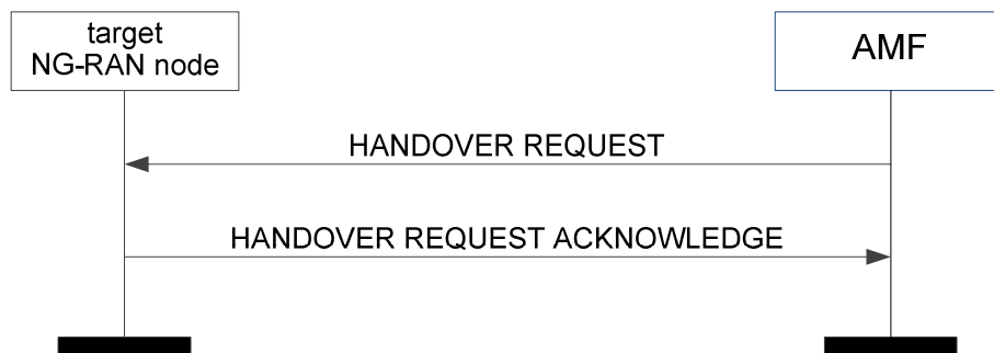
Figure 8.4.2.2-1: Handover resource allocation: successful operation
