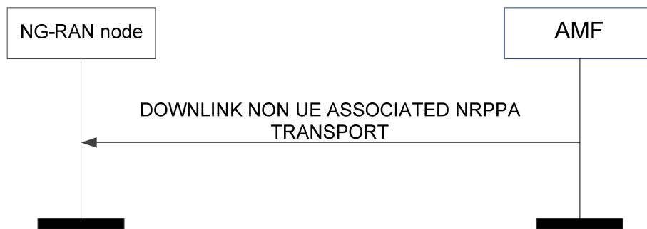
Figure 8.10.2.3-1: Downlink non UE-associated NRPPa transport
