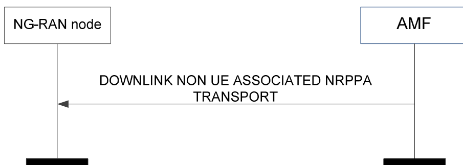
Figure 8.10.2.3-1: Downlink non UE-associated NRPPa transport
