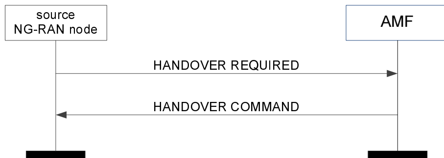
Figure 8.4.1.2-1: Handover preparation: successful operation
