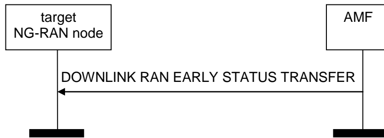
Figure 8.4.10.2-1: Downlink RAN Early Status Transfer
