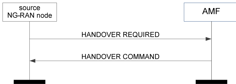
Figure 8.4.1.2-1: Handover preparation: successful operation
