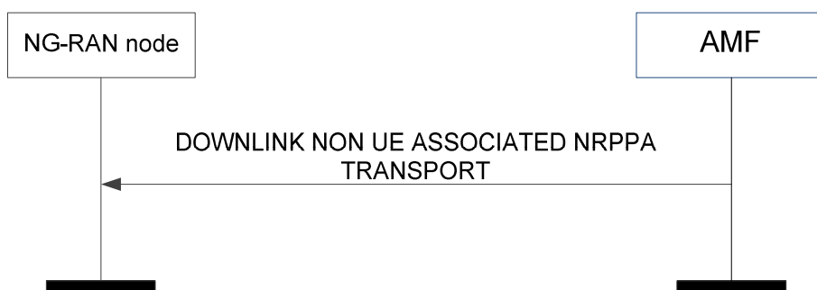
Figure 8.10.2.3-1: Downlink non UE-associated NRPPa transport
