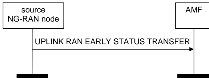
Figure 8.4.9.2-1: Uplink RAN Early Status Transfer
