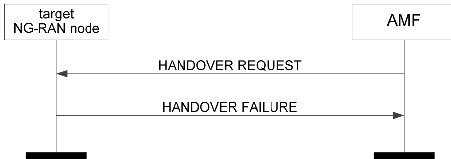
Figure 8.4.2.3-1: Handover resource allocation: unsuccessful operation
