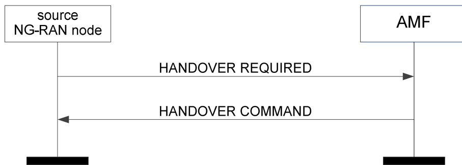
Figure 8.4.1.2-1: Handover preparation: successful operation
