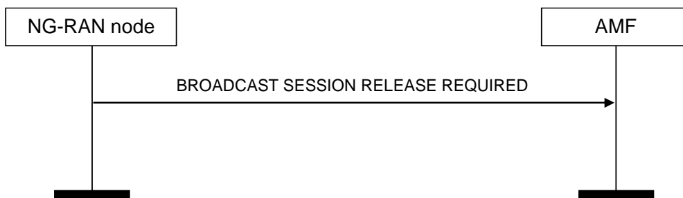
Figure 8.17.4.2-1: Broadcast Session Release Required, successful operation.
