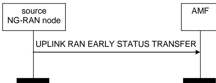
Figure 8.4.9.2-1: Uplink RAN Early Status Transfer
