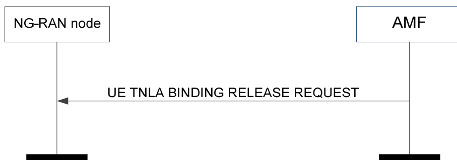
Figure 8.13.1.2-1: UE TNLA binding release request
