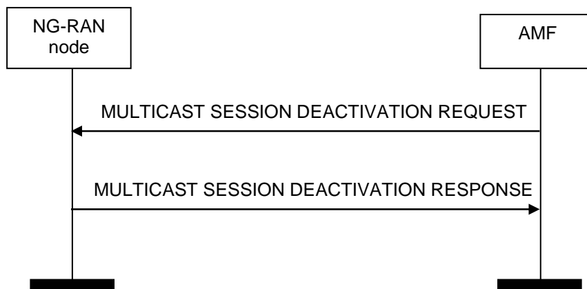
Figure 8.18.4.2-1: Multicast Session Deactivation, successful operation.
