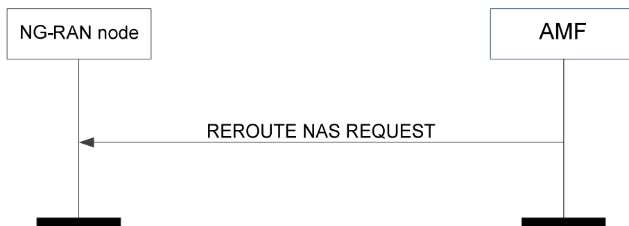
Figure 8.6.5.2-1: Reroute NAS request
