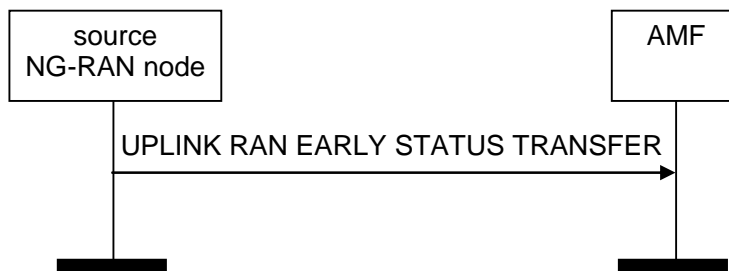
Figure 8.4.9.2-1: Uplink RAN Early Status Transfer
