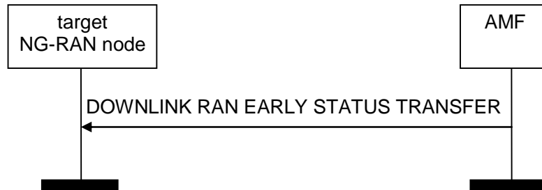
Figure 8.4.10.2-1: Downlink RAN Early Status Transfer
