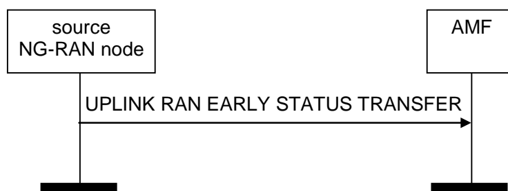
Figure 8.4.9.2-1: Uplink RAN Early Status Transfer
