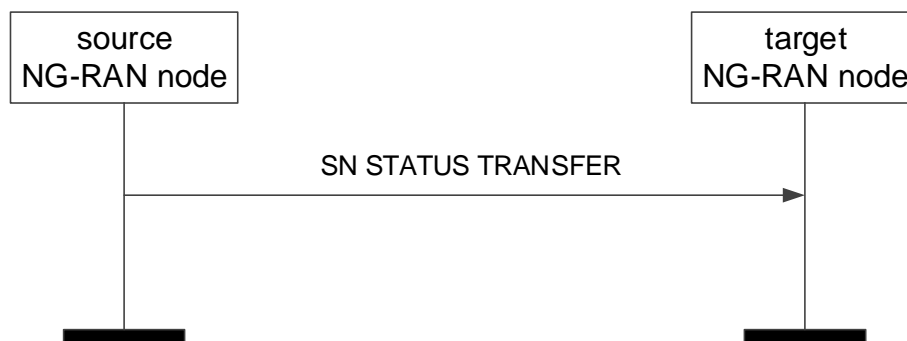
Figure 8.2.2.2-1: SN Status Transfer, successful operation
