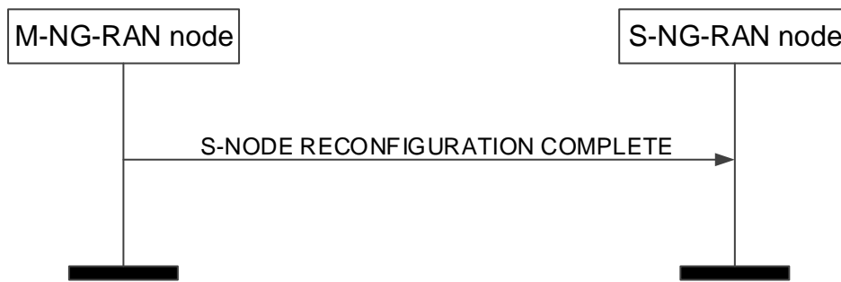
Figure 8.3.2.2-1: S-NG-RAN node Reconfiguration Complete procedure, successful operation.
