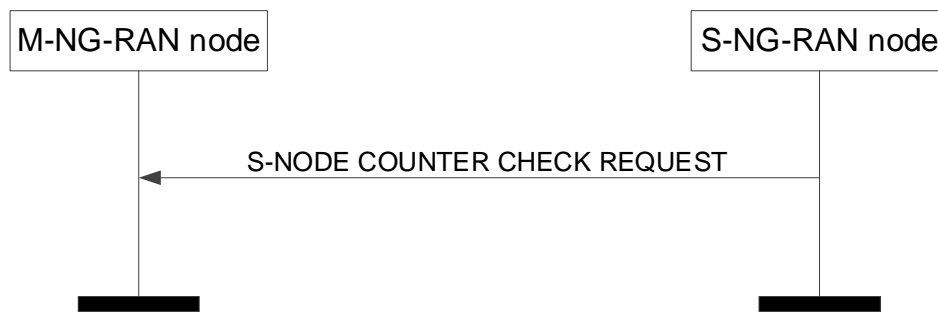
Figure 8.3.8.2-1: S-NG-RAN node Counter Check procedure, successful operation.
