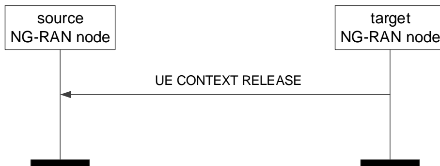
Figure 8.2.7.2-1: UE Context Release, successful operation for handover
