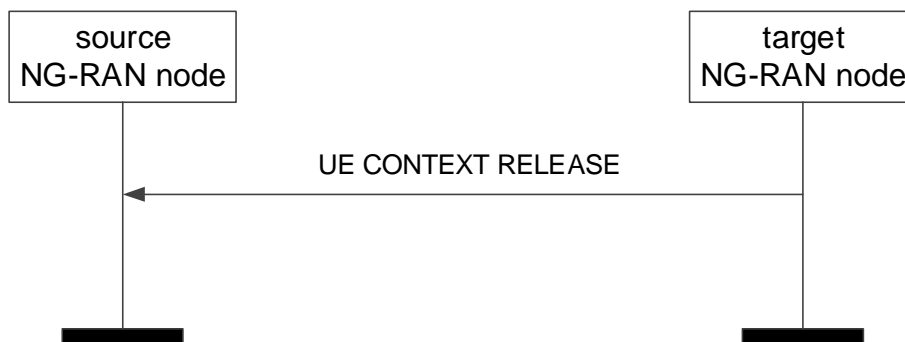
Figure 8.2.7.2-1: UE Context Release, successful operation for handover
