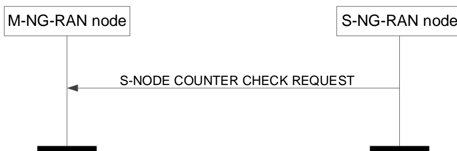
Figure 8.3.8.2-1: S-NG-RAN node Counter Check procedure, successful operation.
