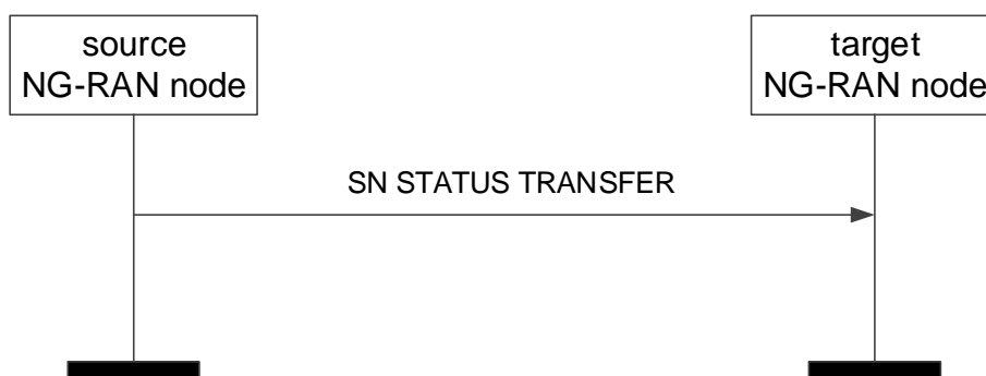
Figure 8.2.2.2-1: SN Status Transfer, successful operation
