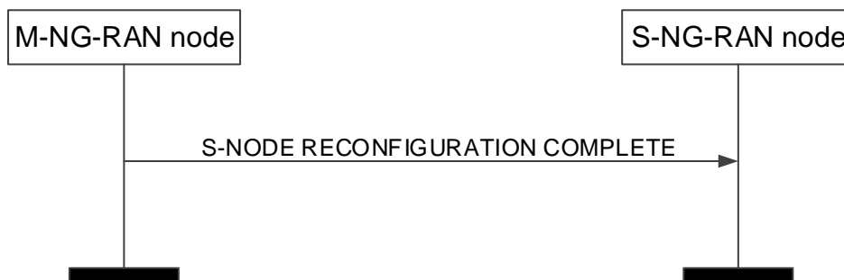
Figure 8.3.2.2-1: S-NG-RAN node Reconfiguration Complete procedure, successful operation.
