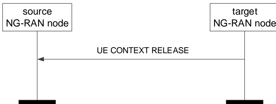
Figure 8.2.7.2-1: UE Context Release, successful operation for handover
