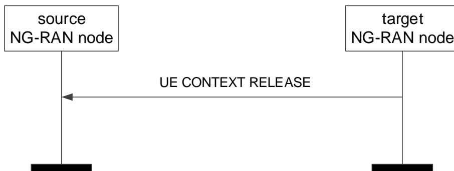
Figure 8.2.7.2-1: UE Context Release, successful operation for handover
