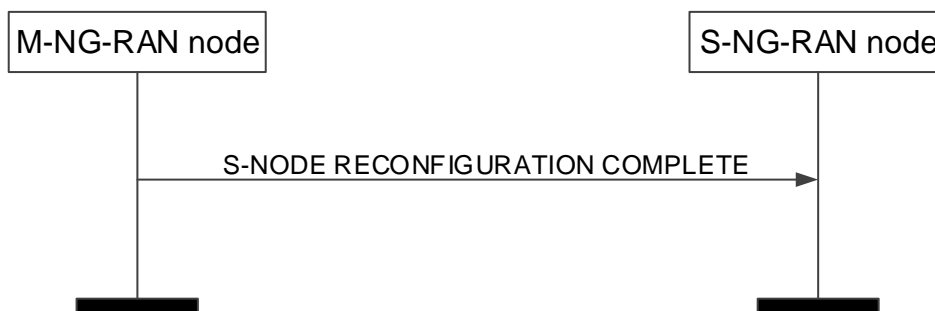
Figure 8.3.2.2-1: S-NG-RAN node Reconfiguration Complete procedure, successful operation.
