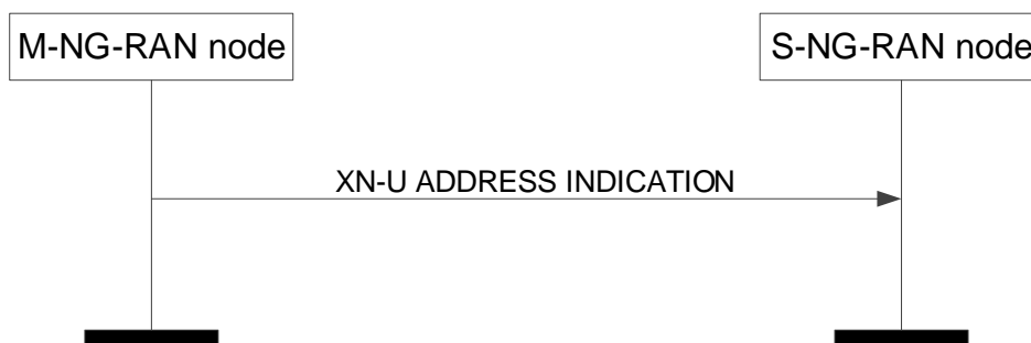
Figure 8.2.6.2-2: Xn-U Address Indication, successful operation for MR-DC with 5GC
