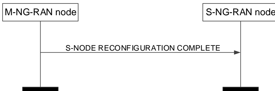
Figure 8.3.2.2-1: S-NG-RAN node Reconfiguration Complete procedure, successful operation.
