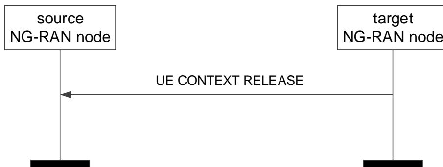
Figure 8.2.7.2-1: UE Context Release, successful operation for handover
