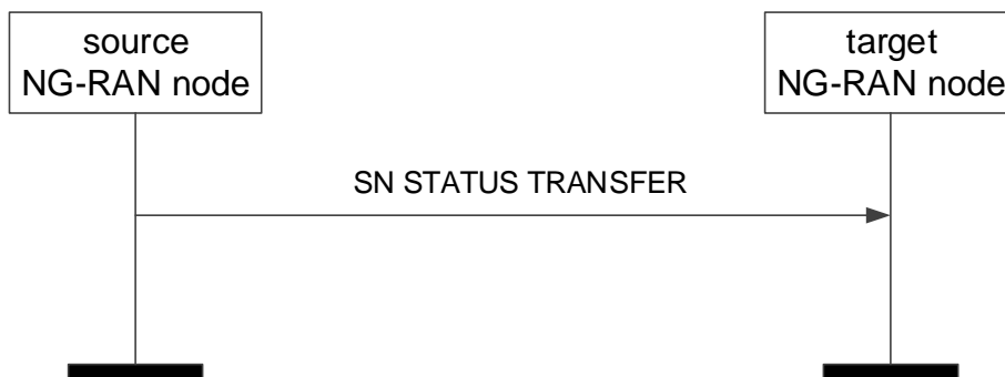
Figure 8.2.2.2-1: SN Status Transfer, successful operation
