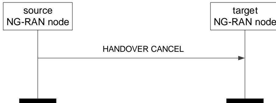
Figure 8.2.3.2-1: Handover Cancel, successful operation
