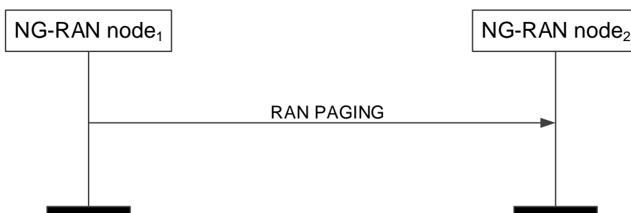
Figure 8.2.5.2-1: RAN Paging: successful operation
