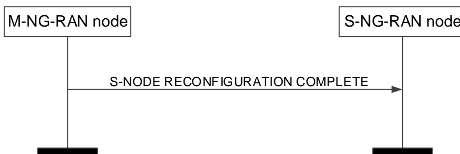
Figure 8.3.2.2-1: S-NG-RAN node Reconfiguration Complete procedure, successful operation.
