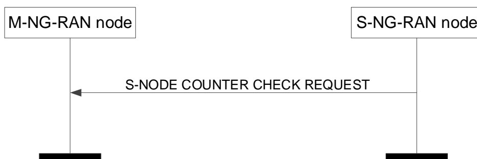
Figure 8.3.8.2-1: S-NG-RAN node Counter Check procedure, successful operation.
