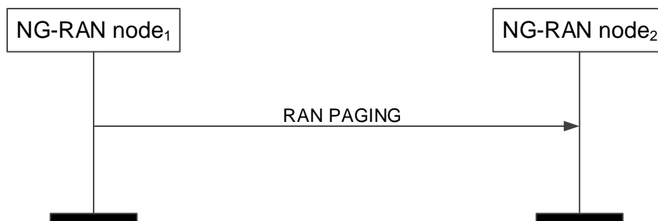
Figure 8.2.5.2-1: RAN Paging: successful operation
