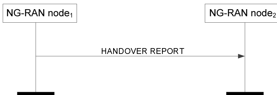
Figure 8.4.8.2-1: Handover Report, successful operation
