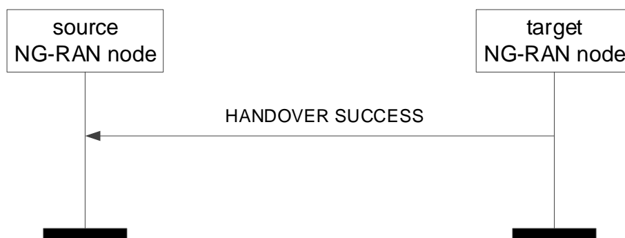
Figure 8.2.8.2-1: Handover Success, successful operation
