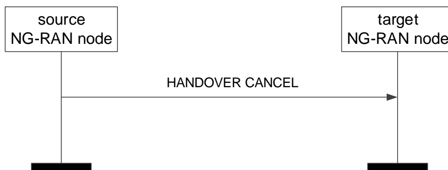
Figure 8.2.3.2-1: Handover Cancel, successful operation
