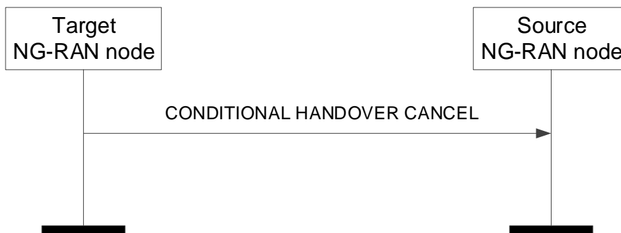
Figure 8.2.9.2-1: Conditional Handover Cancel, successful operation
