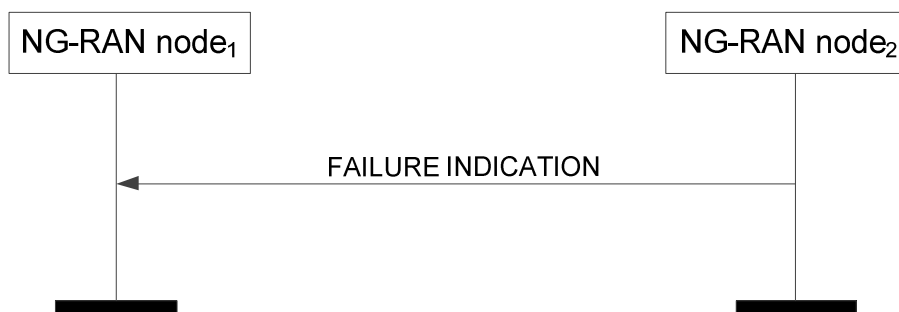
Figure 8.4.7.2-1: Failure Indication, successful operation
