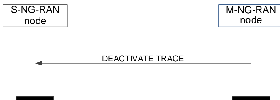
Figure 8.3.15.2-1: Deactivate Trace, successful operation
