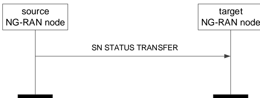
Figure 8.2.2.2-1: SN Status Transfer, successful operation
