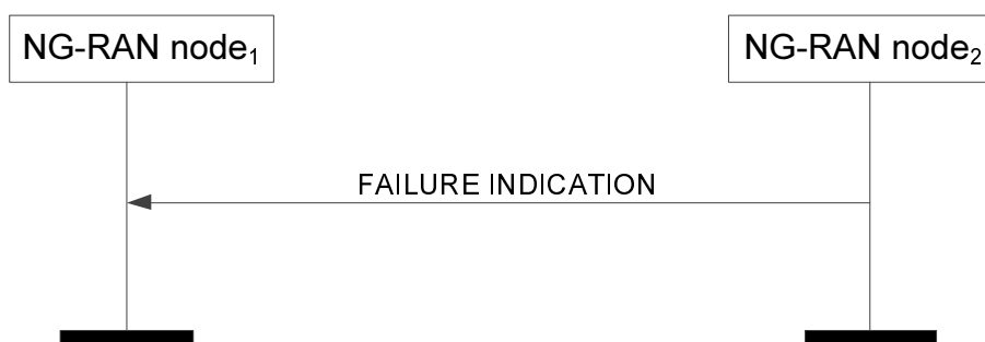
Figure 8.4.7.2-1: Failure Indication, successful operation
