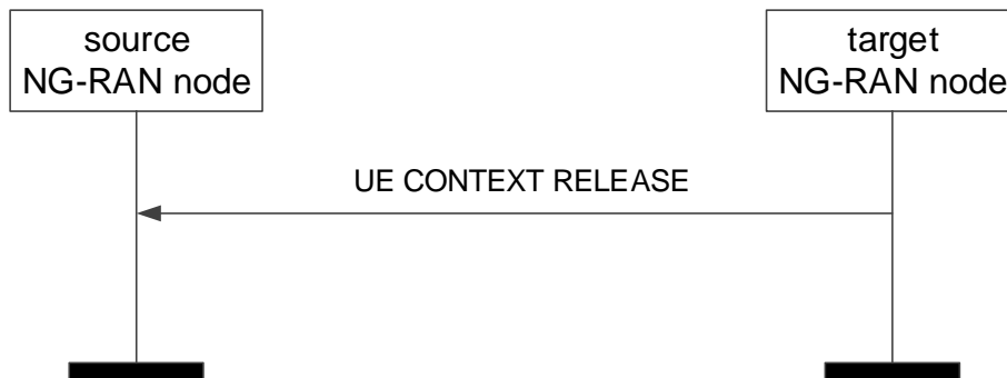
Figure 8.2.7.2-1: UE Context Release, successful operation for handover
