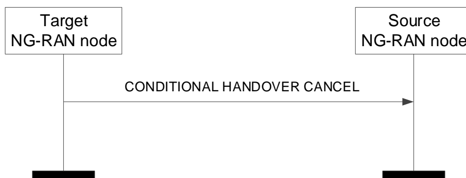
Figure 8.2.9.2-1: Conditional Handover Cancel, successful operation
