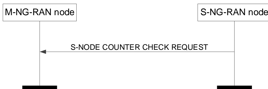
Figure 8.3.8.2-1: S-NG-RAN node Counter Check procedure, successful operation.
