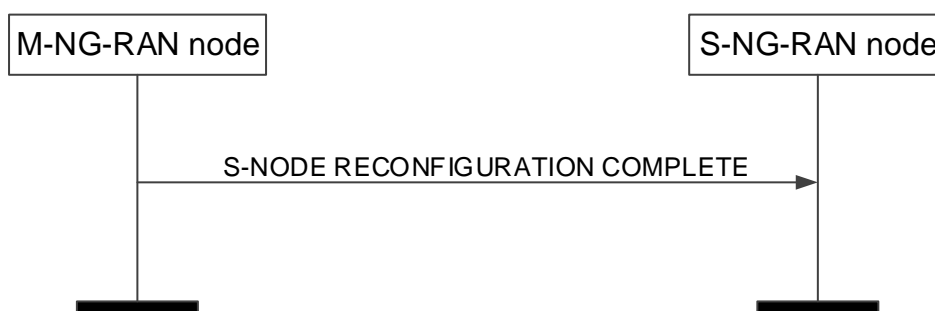
Figure 8.3.2.2-1: S-NG-RAN node Reconfiguration Complete procedure, successful operation.
