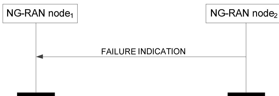
Figure 8.4.7.2-1: Failure Indication, successful operation
