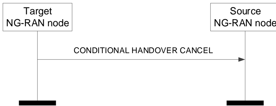
Figure 8.2.9.2-1: Conditional Handover Cancel, successful operation
