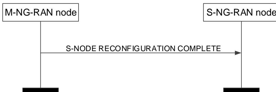
Figure 8.3.2.2-1: S-NG-RAN node Reconfiguration Complete procedure, successful operation.
