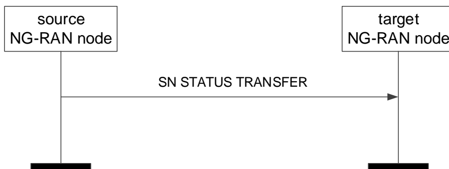
Figure 8.2.2.2-1: SN Status Transfer, successful operation
