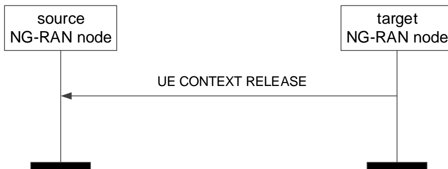
Figure 8.2.7.2-1: UE Context Release, successful operation for handover
