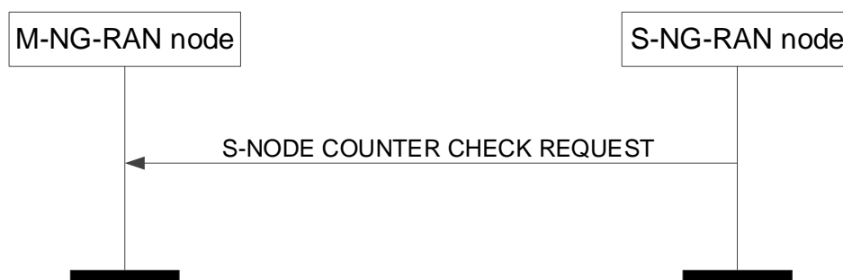
Figure 8.3.8.2-1: S-NG-RAN node Counter Check procedure, successful operation.
