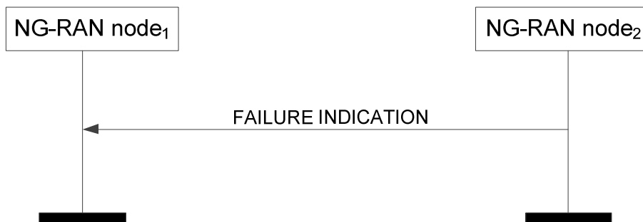
Figure 8.4.7.2-1: Failure Indication, successful operation
