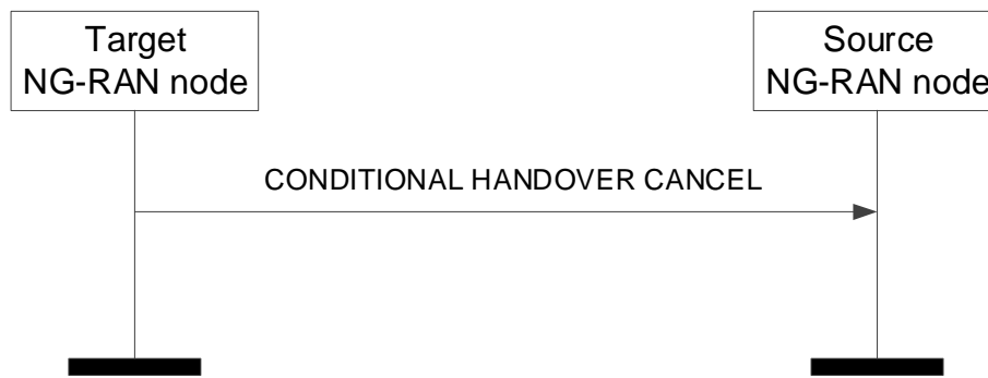
Figure 8.2.9.2-1: Conditional Handover Cancel, successful operation
