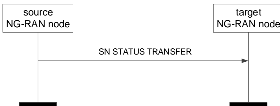
Figure 8.2.2.2-1: SN Status Transfer, successful operation
