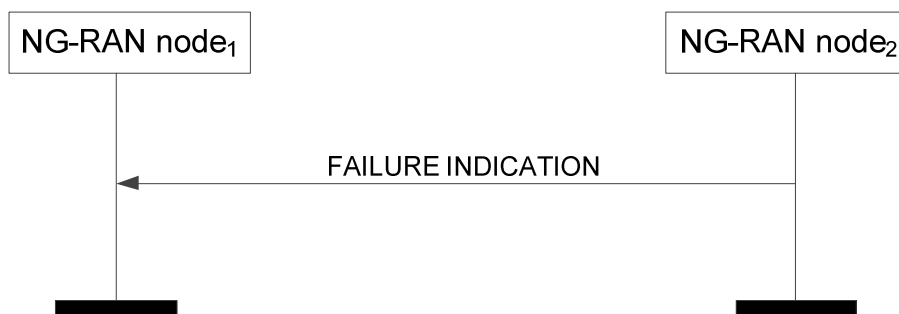
Figure 8.4.7.2-1: Failure Indication, successful operation
