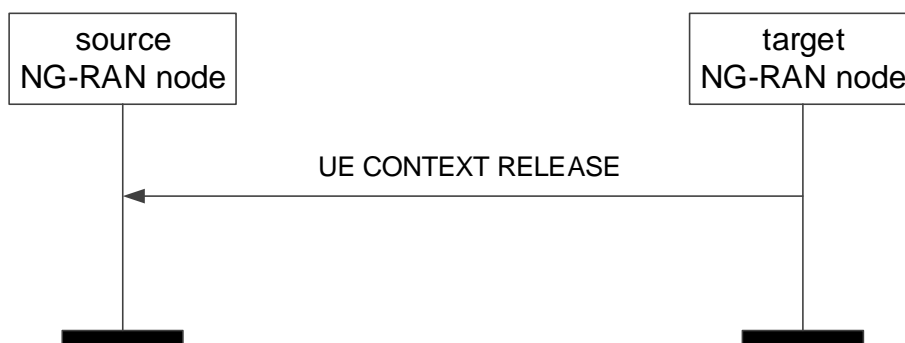
Figure 8.2.7.2-1: UE Context Release, successful operation for handover
