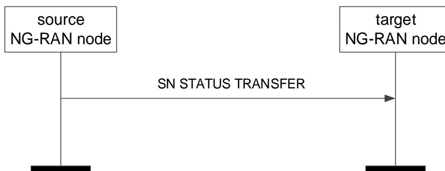
Figure 8.2.2.2-1: SN Status Transfer, successful operation
