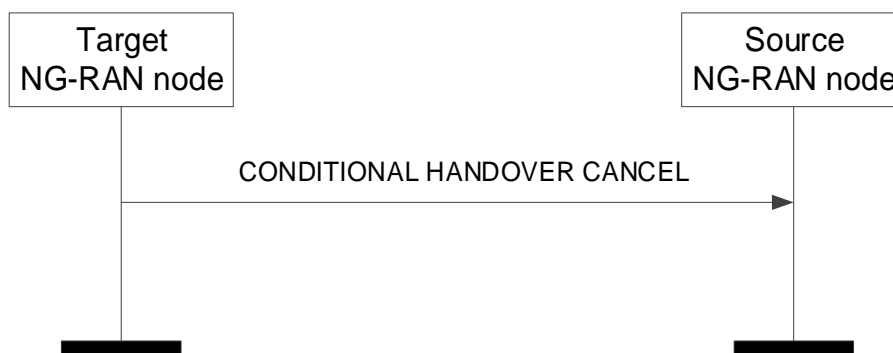
Figure 8.2.9.2-1: Conditional Handover Cancel, successful operation
