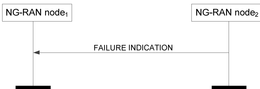
Figure 8.4.7.2-1: Failure Indication, successful operation
