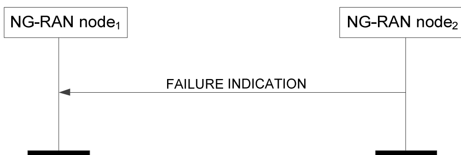
Figure 8.4.7.2-1: Failure Indication, successful operation
