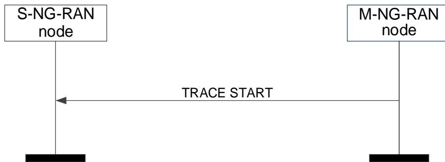
Figure 8.3.14.2-1: Trace Start, successful operation
