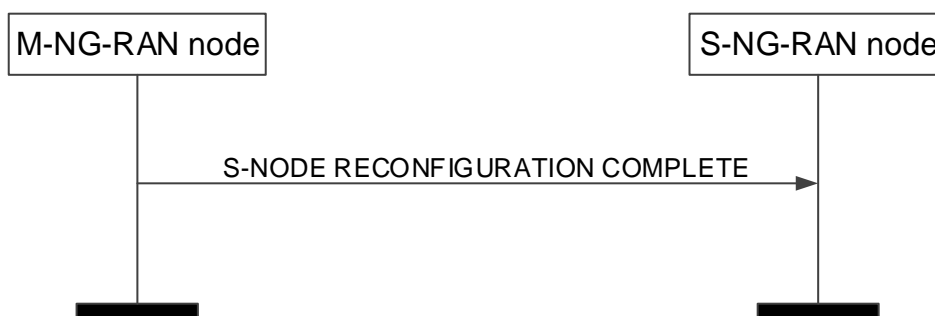
Figure 8.3.2.2-1: S-NG-RAN node Reconfiguration Complete procedure, successful operation.
