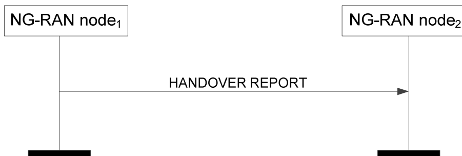
Figure 8.4.8.2-1: Handover Report, successful operation
