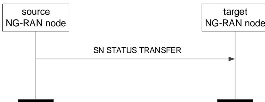
Figure 8.2.2.2-1: SN Status Transfer, successful operation
