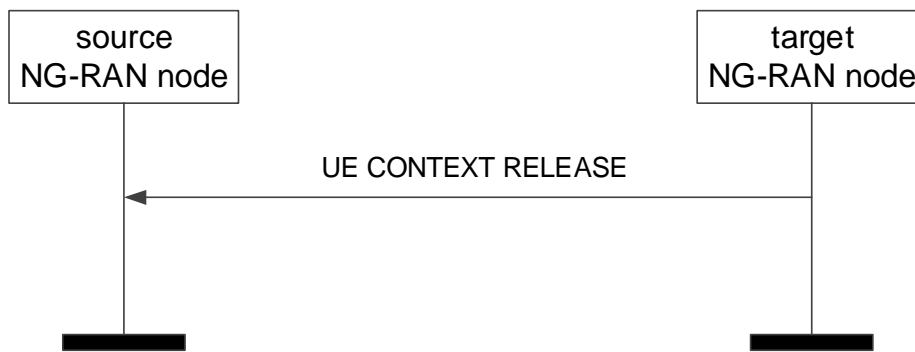
Figure 8.2.7.2-1: UE Context Release, successful operation for handover
