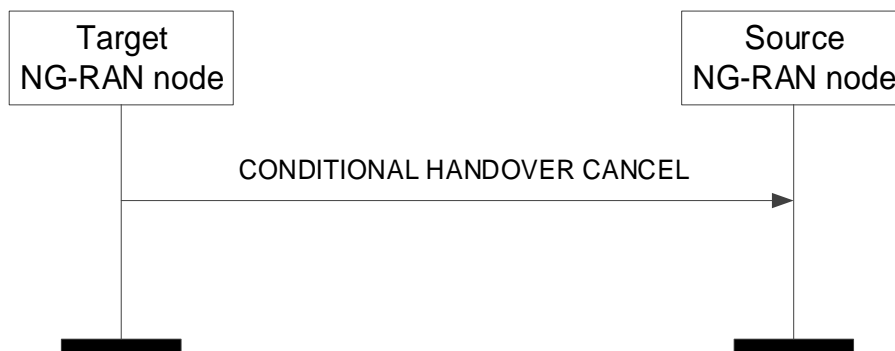
Figure 8.2.9.2-1: Conditional Handover Cancel, successful operation
