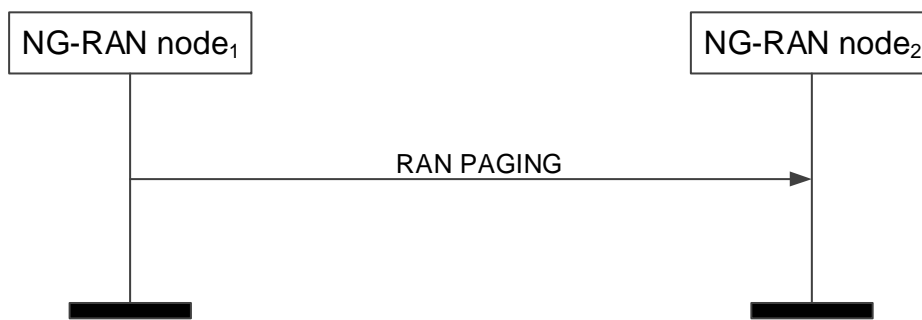
Figure 8.2.5.2-1: RAN Paging: successful operation
