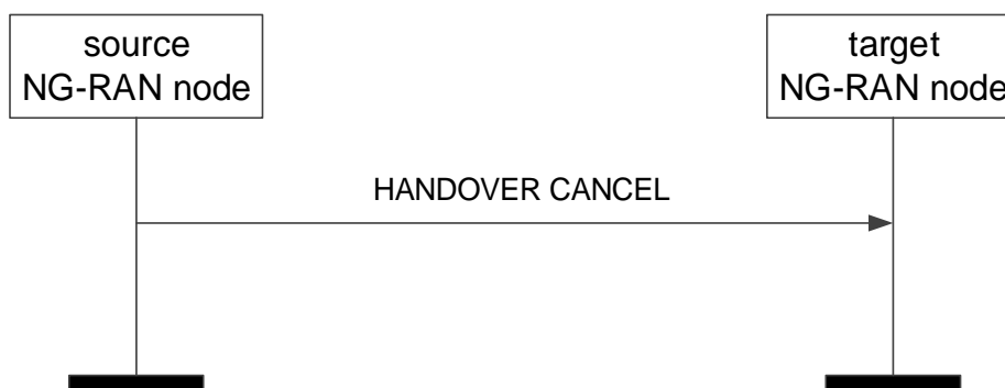
Figure 8.2.3.2-1: Handover Cancel, successful operation
