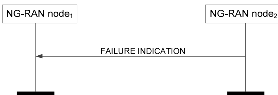
Figure 8.4.7.2-1: Failure Indication, successful operation
