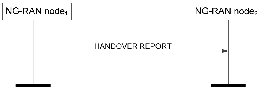
Figure 8.4.8.2-1: Handover Report, successful operation
