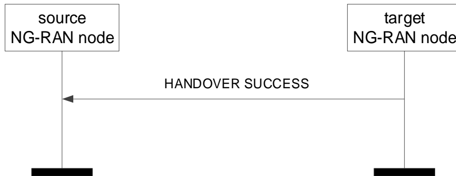
Figure 8.2.8.2-1: Handover Success, successful operation
