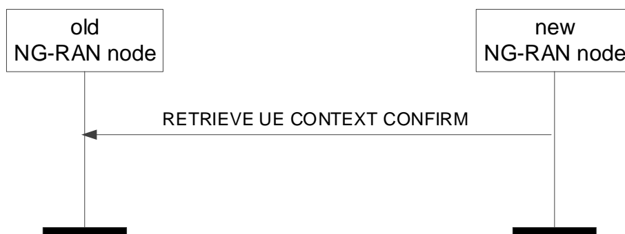
Figure 8.2.12.2-1: Retrieve UE Context Confirm, successful operation
