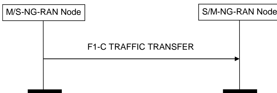
Figure 8.5.1.2-1: F1-C Traffic Transfer procedure, successful operation
