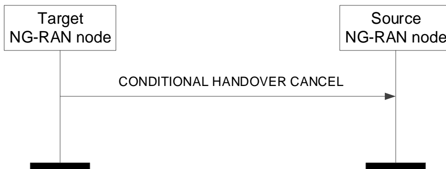
Figure 8.2.9.2-1: Conditional Handover Cancel, successful operation
