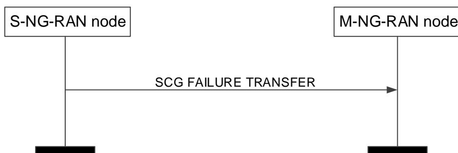
Figure 8.3.18.2-1: SCG Failure Information Transfer, successful operation
