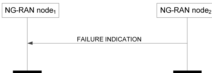
Figure 8.4.7.2-1: Failure Indication, successful operation
